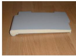
hard foam filling of hollow body
