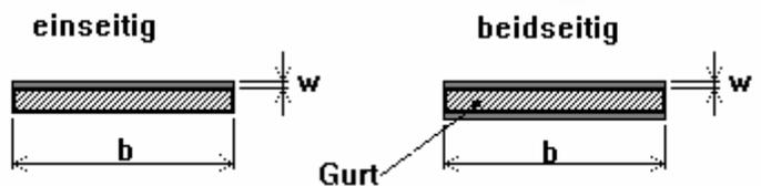
Advantage: excellent flexibility whilst offering good protection against webbing abrasion as well as better skid resistance in comparison to **STOBIPREG** PU spray coatings.
